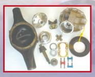
9" Diff Components Gear sets 3-1 to 7.33 - 1Spools, Housing, Bearing Kits, Yokes, U Joints, Complete Custom 9" Diffs new.
